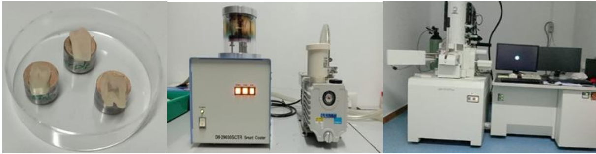
Fig 3: a) Sectioned samples mounted on aluminium stubs b) Geo gold sputter coater c) Scanning electron microscopy.
